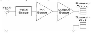
Ultra Short Signal path Careful attention has been paid to the signal path within the amplifier. It is ultra short, guarded by ground planes where necessary and carefully routed to avoid contamination from power supply and high current bearing sections.
