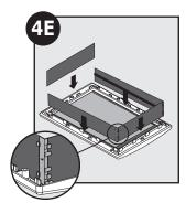
**4E** Snap uncut edge (side with one rib) of assembled core covers inside bottom and side tabs of interior frame (frame with 2 flaps). The bottom core cover should be at bottom of interior frame. Weather strips and ribbed sides (uncut edges) should face flap. Snap the uncut edge (side with one rib) of top core cover inside top tabs of interior frame. Uncut edge (side with one rib) of top core cover should face flap. Core covers may need trimming to meet at corners.
