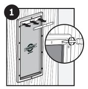
To replace the insulated flap, remove flap screws and flap support from top of pet door frame.
