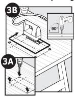
**3A** Drill  $\frac{1}{2}$ " holes in inside corners of drawn template. These will be the pilot holes for the saw blade.
