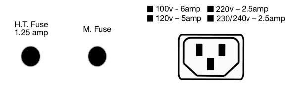
**Warning:** To reduce risk of fire or electric shock, replace fuse with same type and rating only. Do not expose unit to rain or moisture.
