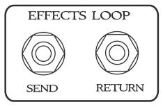
People sometimes inquire about the lack of an effects send. There is one. When the loop is engaged, each Volume control becomes that Volume/Gain's effects send. So, when on the clean channel with the loop engaged, the Volume control on the clean channel becomes the effects send. When on Channel 2, Volume/Gain A, that Volume control becomes 2A's effects send, and so on. So if you're clipping your effects, that is the control to reach for.
