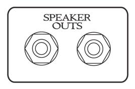
If you are using two speaker cabinets, you should reduce the impedance to half that of the impedance of the cabinets. For example, if you are using two 16ohm cabinets, your impedance selector should be set to 8ohms, not 16 (if you were using only one 16ohm cab, you'd set the impedance selector to 16). So, for example:
