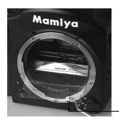
The black mark on the mask must be orientated to the left front corner of the bracket.
