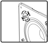
**9.** Adjust tap switch to proper setting. Switch is preset to the 8-ohm mode.
