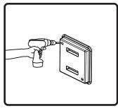
**5.** Insert speaker in hole. Tighten the two clamping screws. **DO NOT OVERTIGHTEN**.
