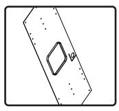
**1.** Nail or screw bracket to studs.
