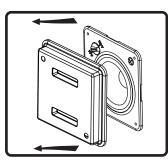
**6.** Remove paint mask unless painting is required. In that case, follow steps 7-10 when painting is complete.
