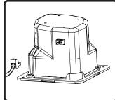
**3.** Connect Euroblock to speaker wires, and connect to speakers.
