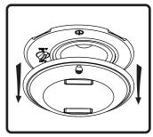
8. Remove paint mask unless painting is required. In that case, follow steps 9-12 when painting is complete.
