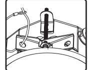
6. If required, attach seismic restraint system to the sheet-metal tab on the rear panel of the speaker, then to reinforced structure (safety cable not included).
