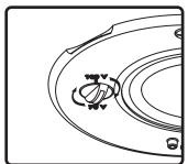
9. Adjust tap switch to proper setting. Switch is preset to the 80hm mode.
