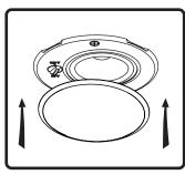
11. Align tabs on snap-fit grille with slots in baffle,
