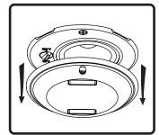
**7.** Remove paint mask unless painting is required. In that case, follow steps 8-11 when painting is complete.
