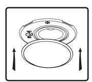
**10.** Align tabs on snap-fit grille with slots in baffle, gently press grille into place.
