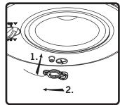
**10.** Attach grille safety clip by placing the large end of the clip over snap-fit post (1), gently press grille into place. then sliding clip until small end snaps into place around post (2).
