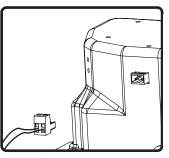
**4.** Connect Euroblock to speaker wires, and connect to speakers.
