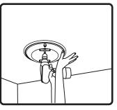
7. Insert speaker into mounting hole. Tighten both screws on the baffle face to actuate the mounting wings. DO NOT OVERTIGHTEN.
