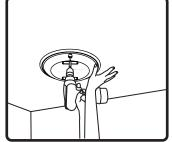
6. Insert speaker into mounting hole with paint mask in place. Tighten both screws on the baffle face to actuate the mounting wings. Firmly secure both screws, DO NOT OVERTIGHTEN.
