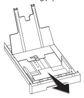
4 Removing the tape in the paper tray which was used for transportation purposes.
