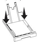
**8** Push the paper tray into the device all the way to the stopping point.
