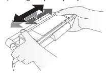
**7 Only after** completely pull off the protection strip located on the left side of the cartridge.
