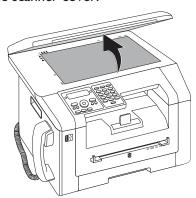
**2** Lay the document onto the scanner glass with the written side down.
