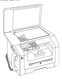
3 Align the document with the rear left corner of the scanner glass (arrow marks). The markings on the scanner border for the A4 and A5 formats will help you to position the document correctly.
