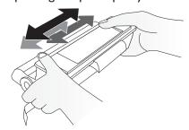
6 Only after completely pull off the protection strip located on the left side of the cartridge.
