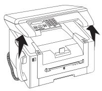
2 Open the device by lifting the device cover forwards
