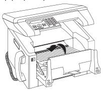
7 Place the toner cartridge into your device. The cartridge should snap securely into position.
