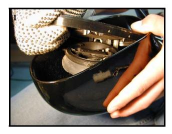
While using sturdy gloves, position your fingers behind the outboard edge of the mirror. Pull back on the mirror to dislodge it from the center hub and remove the mirror from the housing.
