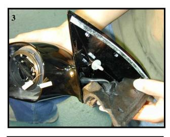
Carefully peel back the foam insulation on the mirror housing sail.
