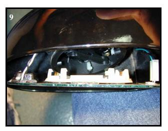
Tuck the wires toward the back of the mirror housing. Align the *Signal*® mirror over the center hub of the mirror housing and firmly press the mirror into the housing until it snaps into position.
