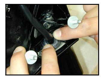
Pull the rubber grommet back out from the mirror housing and reposition.
