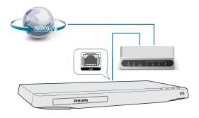
For Wi-Fi, connect a Philips Wi-Fi USB adapter (named WUB1110) to the •  $\hookrightarrow$  (USB) connector on the front panel of this player.
