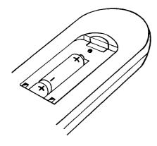
The remote control and its batteries are packed separately in the original video recorder packaging. You must install the batteries in the remote control before use - described in the following section.
