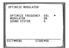
Tune in the TV set to the new modulator frequency (channel 21 - 69) shown in the video recorder display.
