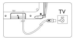
2 Connect the DC plug to the antenna and the power supply to a 100-240V AC outlet.
