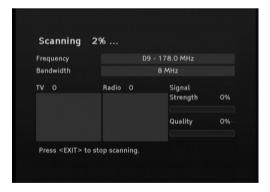
Note: By pressing the **EXIT button**, you can stop the scan mode at any time.
