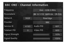
4 Adjust your antenna so that the two specifications signal strength and signal quality display a preferably high value. Note: Depending on your antenna, you can possibly also carry out settings on your antenna.
