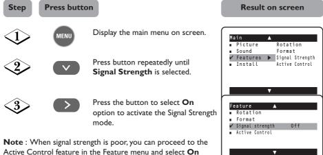
Active Control feature in the Feature menu and select **On** option to automatically adjust settings for optimal picture quality (Refer to section on "Using the Active Control").
