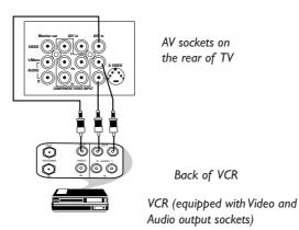
You can view the playback of VCR tapes (Video Disc players, camcorders, etc.) by using the AUDIO and VIDEO INPUT sockets on the rear of the TV.
