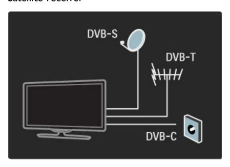
Next to the DVB-T and DVB-C reception, this TV has a built-in satellite DVB-S receiver. You can connect a satellite dish antenna and receive digital satellite channels.
