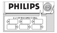
Make sure you remove the plug from the set and wall socket before inserting batteries.
