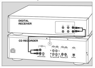
1 For separate playback on the CD player deck, connect a third cable 3 (not supplied) between the ANALOG OUT sockets of the CD recorder and the input sockets of an amplifier e.g. CD, or AUX.
