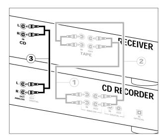
1 For separate playback on the CD player deck, connect a third cable ③ (not supplied) between the ANALOG OUT sockets of the CD recorder and the input sockets of an amplifier e.g. CD, or AUX.
