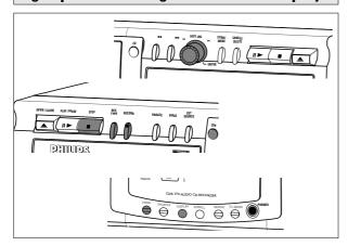
During high speed recording the sound is not audible.
