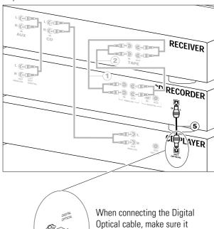
**1** Remove the dust caps from the digital optical connection. (We recommend you save the cap.)
