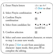
Enter the pinyin letters accordingly. Press once on the key corresponding to the pinyin letter without having to consider its position on the key. Pinyin input method will automatically select and list all possible combinations for you to select.
