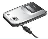
The battery symbol indicates the state of charge. During charging, the charge indicators will scroll; it takes around 2.5 hours to fully charge the battery. When all the scroll bars are steady, the battery is fully charged. You can then disconnect the charger. Depending on the network and condition of use, talk time and stand-by time can go up to 8.5 hours\* and 30 days\* respectively.
