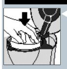
Place a paper filter (type 1x4 or no.4) in the brew basket. Do not forget to fold the sealed edges of the filter.
