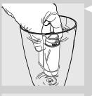
2 Remove the "INTENZA+" water filter from its packaging, immerse it vertically (with the opening positioned upwards) in cold water and gently press the sides so as to let the air bubbles out.
