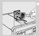
**5** Lift the pre-ground coffee compartment lid and add one scoop of pre-ground coffee to the compartment. Use only the measuring scoop supplied with the machine. Then close the pre-ground coffee compartment lid.
