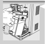
1 Slightly tilt the milk carafe and then insert the front part into the machine.
