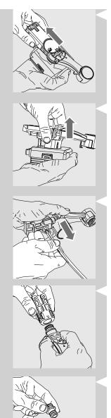
5 Remove the connector which is in contact with the machine.
