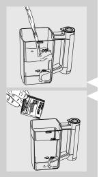
5 Fill the milk carafe with fresh drinking water up to the MAX level. Pour one milk cleaner bag into the milk carafe and let it dissolve completely.
