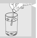
1 Immerse the water hardness test strip provided with the machine in water for 1 second.
