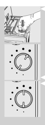
2 Press and turn the grinder adjustment knob one notch at a time. You will taste the difference after brewing 2-3 cups of espresso.
