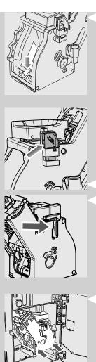
8 Gently pull down the lever until it is in contact with the brew group base and the two reference signs on the side of the brew group do match.
