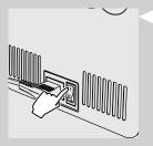
12 Switch the power button to "I" to turn on the machine.
