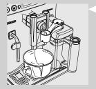
Insert the milk carafe and place the cup under the dispensing spout. Open the milk dispenser by turning it clockwise.
