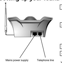
1 On the top side of the base station, connect the telephone cable to the smaller of the sockets and then to the telephone socket in
