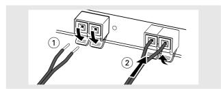
Fully insert the stripped portion of the antenna into the jacks as shown.
