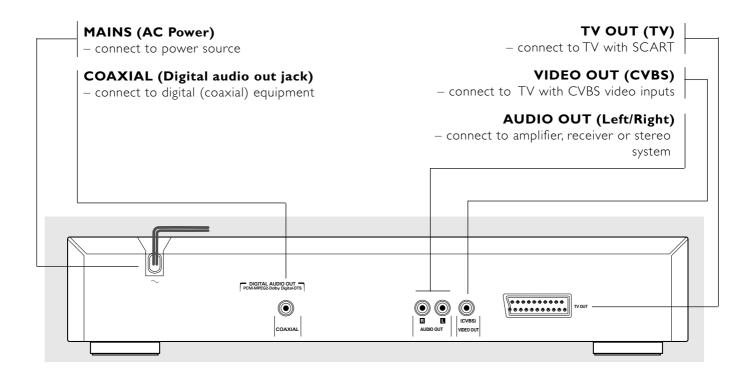
Caution: Do not touch the inner pins of the jacks on the rear panel connectors. Electrostatic discharge may cause permanent damage to the unit.
