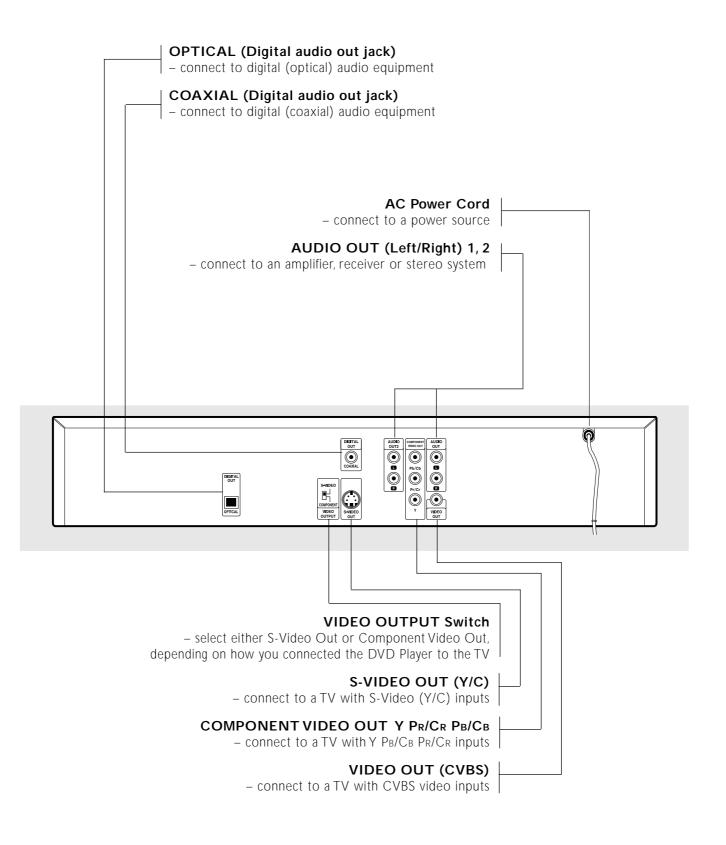
Caution: Do not touch the inner pins of the jacks on the rear panel. Electrostatic discharge may cause permanent damage to the unit.
