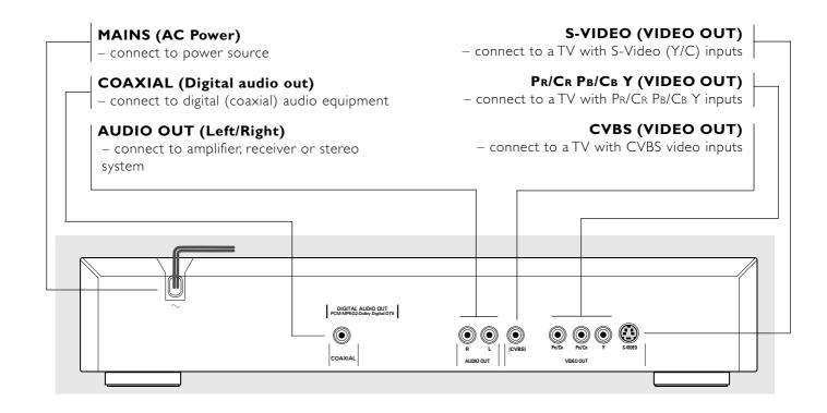
Caution: Do not touch the inner pins of the jacks on the rear panel. Electrostatic discharge may cause permanent damage to the unit.
