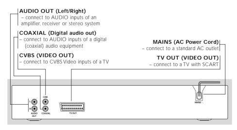
Caution: Do not touch the inner pins of the jacks on the rear panel. Electrostatic discharge may cause permanent damage to the unit.
