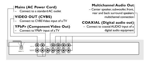
Caution: Do not touch the inner pins of the jacks on the rear panel. Electrostatic discharge may cause permanent damage to the unit.
