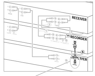
When connecting the Digital Optical cable, make sure it is fully inserted until there is a click.
