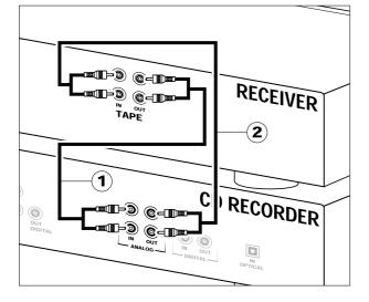
Use the audio cables supplied. Connect the red plugs to the R sockets, and the white plugs to the L sockets.
