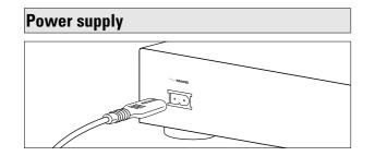
**1** Plug the power cord supplied into the POWER SUPPLY connector on the CD recorder, then into a wall socket.
