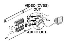
Insert one end of the video (CVBS) cable into the yellow Cinch socket OUT VIDEO (CVBS) at the back of the DVD recorder and the other end into the video input socket (usually yellow) on the TV set (usually labelled 'Video in' or 'AV in'. See TV operating instructions).
