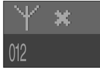
No signal - Channel is not receivable or no equipment is connected to this jack.
