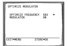
Select the line 'MODULATOR' on the TV screen or 'MDI+' in the display with  $P^+$  or  $P \downarrow -$ .
