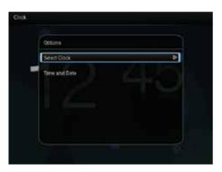
[Select Clock]: Move the joystick left/right to select another clock or calendar to be displayed.  [Time and Date]: Move the joystick up/ down/left/right to set time/date or to select a time/date format. For details, see "Settings" > "Set time and date".
