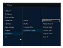
→ If you select [RadiantColor], the PhotoFrame extends the color on the edges of a photo that is smaller than the full screen to fill the screen without black bars or aspect ratio distortion.
