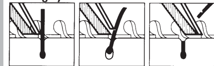
Groove channels beard closer to cutting system
