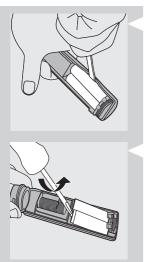
9 Pry the 2 AA-sized cylindrical nickel-cadmium batteries loose by inserting the screwdriver on the sides of the two batteries in the locations shown in the figure.
