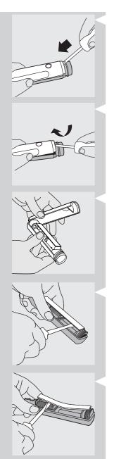
4 Now, insert the screwdriver into the middle slot located on the top front part of the handle as shown and push the blade in as far as it will go.
