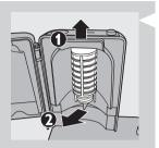
Remove the protective screen in front of the UV light bulb.
