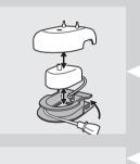
If your model includes the deluxe charger cover and base, the travel charger is pre-installed inside the cover. If you want to shorten the power cord, you can store excess cord in the cord wrap feature built into the charger base.
