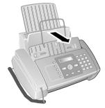
2 Insert paper in the paper feeder. You can insert maximum 100 sheets (A4 · 80 g/m²).
