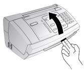
Lock the cover of the device completely into place when opening the device. You could be injured if the cover falls while you are working on the de**3** Grip the rear ink film roll at both the sides and place it next to the front ink film roll.
