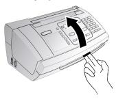
Lock the cover of the device completely into place when opening the device. You could be injured if the cover falls while you are working on the de-
