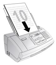
2 Set the desired resolution. You can choose between RESOL.: STANDARD (for documents without special features), RESOL.: FINE (for texts with small print or drawings) and RESOL.: PHOTO (for photos). Press ■. The configured resolution appears on the display. Press ■ again to change the resolution.
