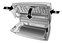
4 Lightly wipe the upper side of the scanner glass (A) and the lower side of the document feeder/scanner film (= white plastic plate) (B) with a cloth.
