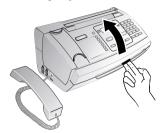
Lock the cover of the device completely into place when opening the device. You could be injured if the cover falls while you are working on the device.
