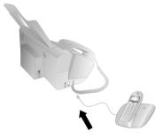
We recommend direct connection to the device because this allows the fax switch to function optimally and to control the additional devices.
