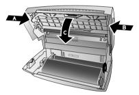
4 Carefully pull the document to the front or to the back out of the device.
