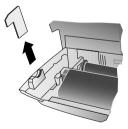
**6** Carefully remove the rubber bands from the new ink film. Make sure that the film is not damaged!
