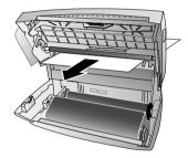
**4** Turn the blue gear wheel forward to tension the ink film. The ink film must not have any creases.
