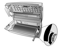
7 Close the device. Insert the paper tray in the opening provided for it behind the paper feeder. Insert paper again.
