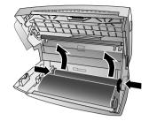
**4** Remove both the rolls from the device. The used ink film cannot be reused.
