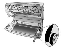
8 Close the device. Insert the paper tray in the opening provided for it behind the paper feeder. Insert paper again.
