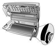
**11** Close the device. Insert the paper tray in the opening provided for it behind the paper feeder. Insert paper again.
