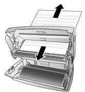
5 Close the scanner cover and the cover of the automatic document feeder. Both the supports must securely snap into place.
