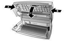
4 Lightly wipe the upper side of the scanner glass (A) and the lower side of the document feeder/scanner film (= white plastic plate) (B) with a cloth.
