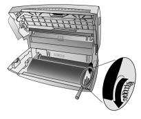
11 Close the device. Insert the paper tray in the opening provided for it behind the paper feeder. Insert paper again.
