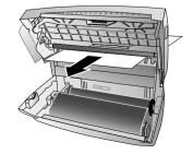
**4** Turn the blue gear wheel forward to tension the ink film. The ink film must not have any creases.
