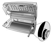
5 Close the device. Insert the paper tray in the opening provided for it behind the paper feeder. Insert paper again.
