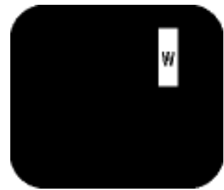
Three adjacent lit subpixels (one white pixel)
