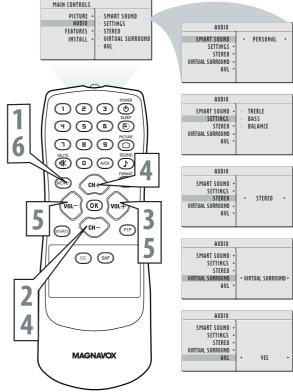
PIP (Picture-in-Picture) feature allows you to call up a subscreen when you are using your TV as a monitor.
