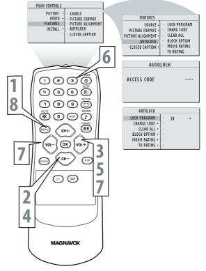
Note: You can block additional channels by using Number buttons to jump to another channel.
