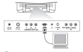
Connect one end of a (male to male) VGA cable to the video card of the computer and the other end to the VGA connector **PC INPUT** at the back of the TV. Fix the connectors firmly with the screws on the plug.
