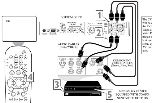
The CVI connection will be dominate over the AV1 in Video Input. When a Component Video Device is connected as described, it is best not to have a video signal connected to the AV1 in Video Input jack.
