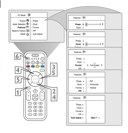
Before using the PIP feature configure the computer for optimum resolution (1024 x 768, 60Hz).
