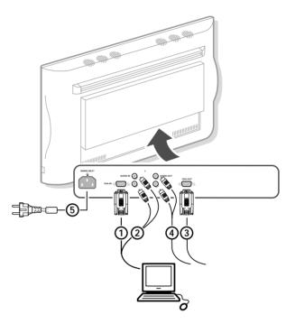
In case of a Multimedia computer, also connect the audio cables to AUDIO OUT R and L 2 next to the VGA OUT connector and to the audio inputs of the second VGA monitor.
