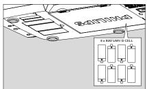
Open the battery compartment and insert 8 batteries, type R-20, UM-1 or D-cells, (preferably alkaline) with the correct polarity as indicated by the "+" and "-" symbols inside the compartment.
