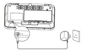
2 Connect the other end of the AC adaptor to the wall outlet.
