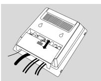
2 Align the side marked PRESS▼ of the stand to the slots at the bottom of the set.
