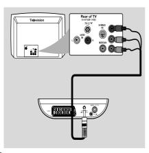
Use component video cables (red/blue/green) to connect the COMPOENT VIDEO OUTPUT (Pr/Cr Pb/CbY) jack to the corresponding Component video input jacks (or labeled as Y Pb/Cb Pr/Cr or YUV) on the TV.
