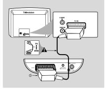
Use the SCART cable (black) to connect the DVD Player's SCART jack (SCART) to the corresponding Scart input jacks on the TV.
