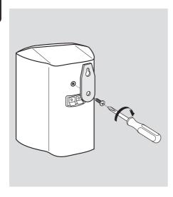
You can choose to hang the speakers on the wall. Attach the supplied bracket firmly to the rear of speakers using the supplied screws. Then mount a screw (not supplied) on the wall where the speaker is to be hung and hook the speaker securely onto the mounted screw.
