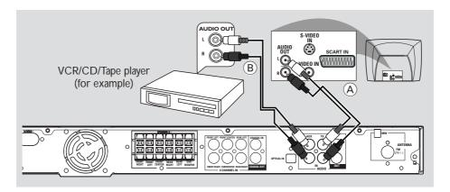
To hear the TV channels through this AV receiver, use the audio cables (white/red) to connect AUDIO IN-TV jacks to the corresponding AUDIO OUT jacks on the TV (see fig (A)).
