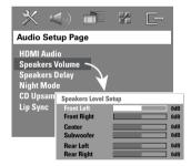
4 Use ◀ ► keys to set the volume level for each speaker (-6dB ~ +6dB) and press OK to confirm.
