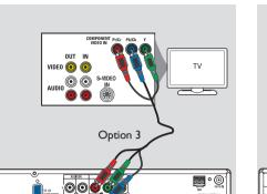
Option 3: Connecting to a Progressive Scan TV or component video input
