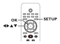
In 'DISC' mode, press SETUP on the remote control.
